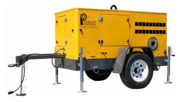
Standard engine features: Safety shutdown switches for low oil pressure and high temperature. Instrument panel with temperature and oil pressure gauge, ampmeter, hourmeter and tachometer. Muffler with rain cap. Engine to pump coupling: SAE5 housing with 7.5" rubber disc drive.
